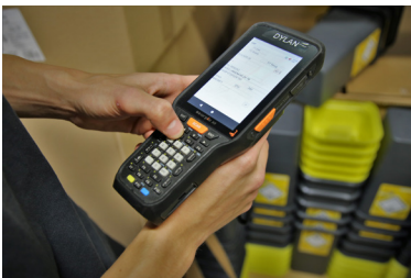
The pistol grip enables practical use and helps reduce the likelihood of the terminals getting lost.
